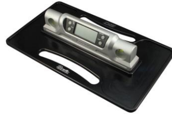
Figure 6: Official measuring device to check saddle inclination
