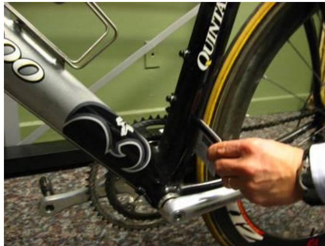
Figure 53: Insertion of a credit card between the wheel and frame to check that a fairing is not present
