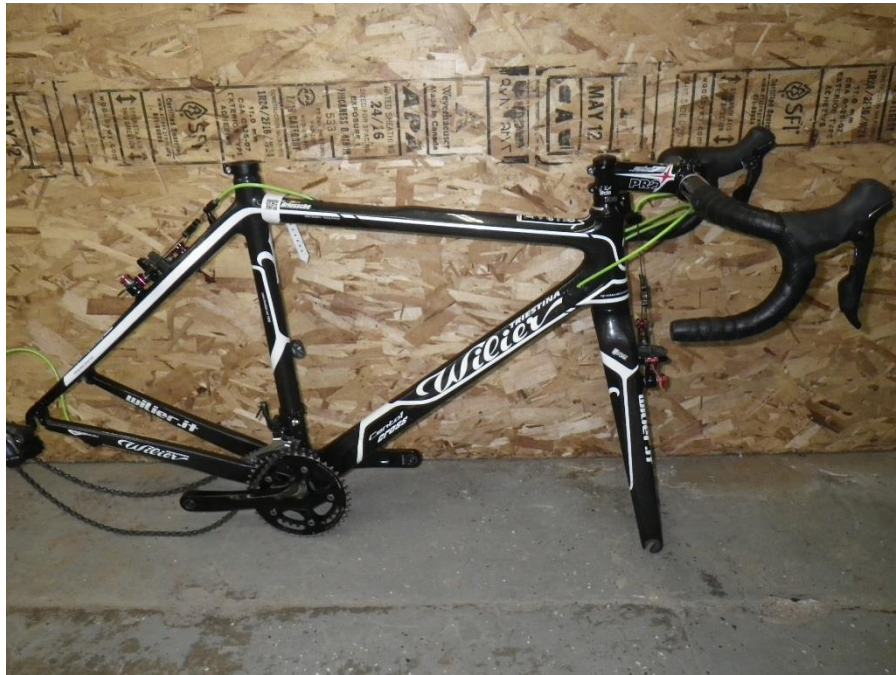
Figure 7: Wilier Cento1 Cross carbon cyclocross frame and fork, with known, bicycle specific motor contained in the seat-tube.
