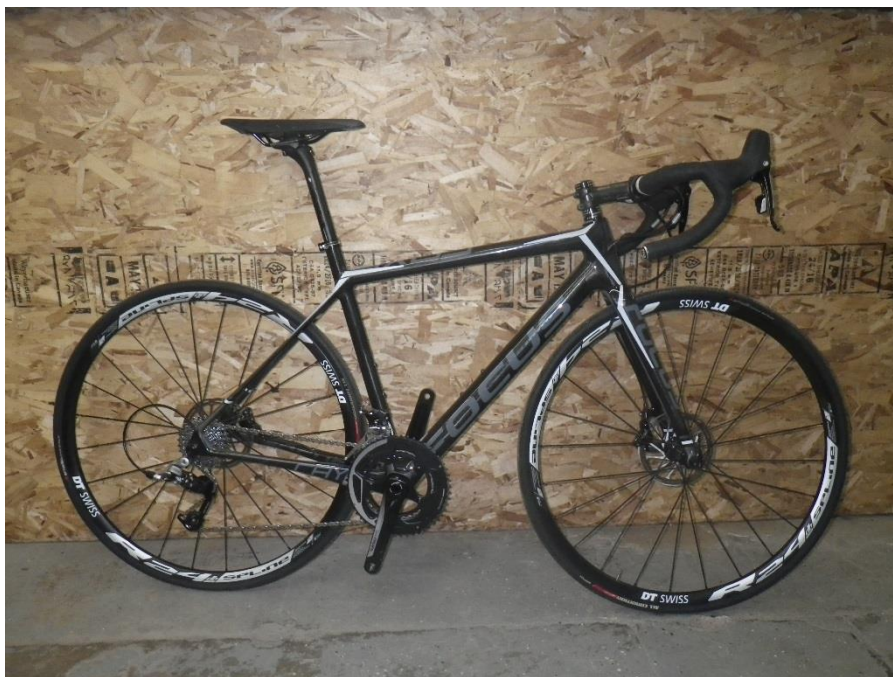
Figure 3: Focus Cayo carbon, small size, SRAM Rival mechanical drivetrain.
