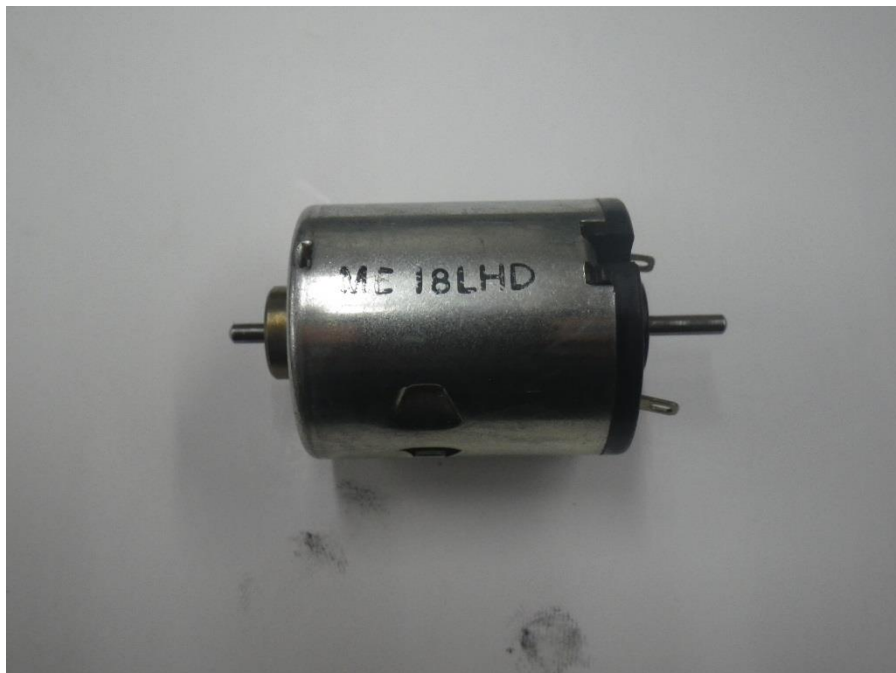
Figure 8: Micromo series M3138U DC micromotor with 6V windings and output power of 19.65 watts.
