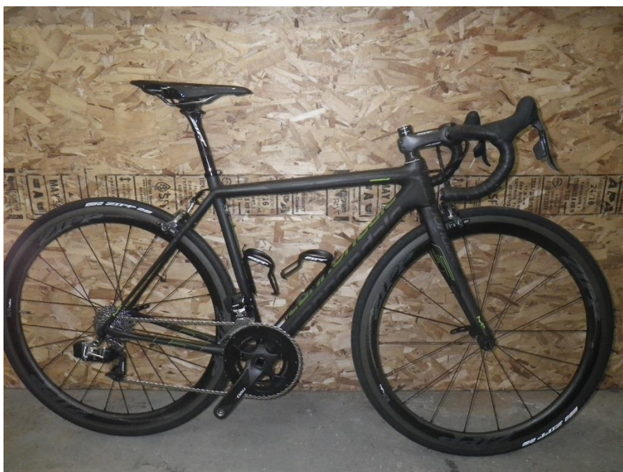
Figure 4: Cannondale Supersix Evo carbon, 48cm, SRAM Red Etap electronic drivetrain.
