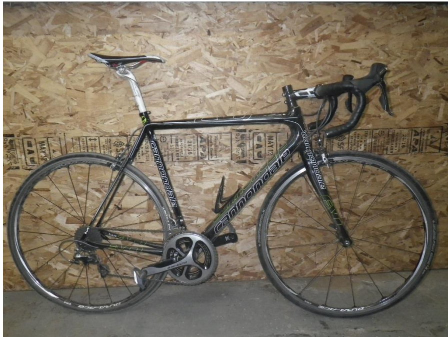
Figure 5: Cannondale Supersix Evo carbon, 56cm, Shimano Dura-ace mechanical drivetrain.
