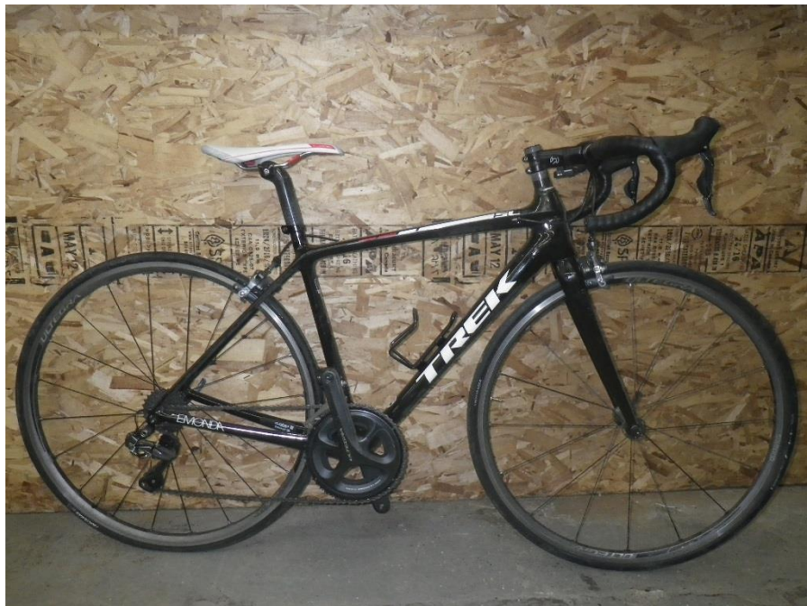
Figure 6: Trek Emonda SL carbon, 50cm, Shimano Ultegra Di2 electronic drivetrain.
